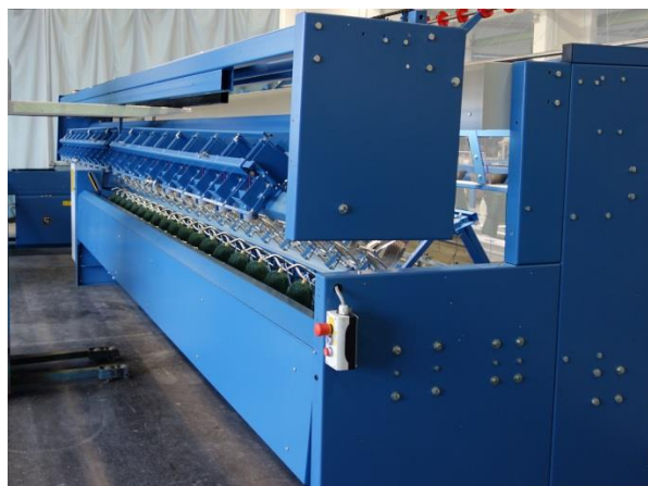
Option: Band magazine unit to retrofit model KA to model RKC for fully-automatic operation (with forklift or crane)
